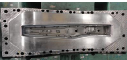
Mold of Company "S" produced from TD1 (DP 980 forming)
